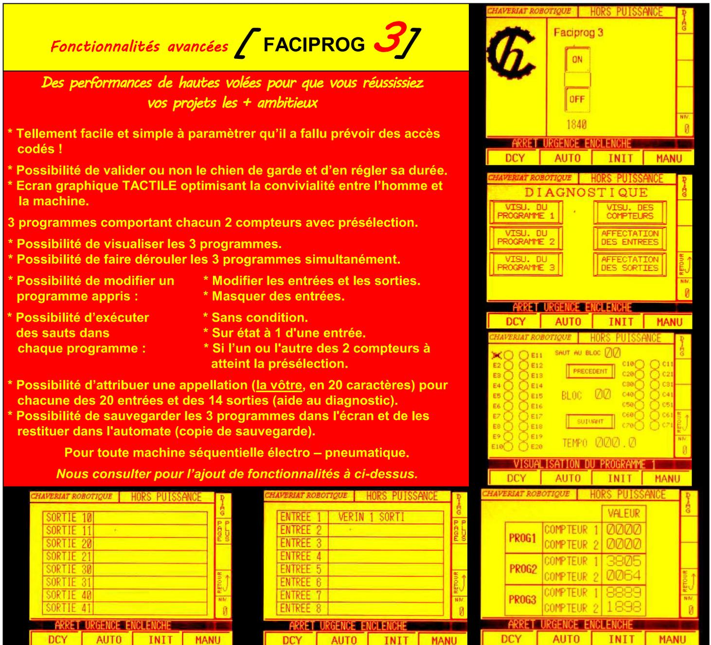
The image displays three screenshots of the FACIPROG 3 control interface. The top screen shows the power status (HORS PUISSANCE) and a large 'ON' button. The middle screen is the 'DIAGNOSTIQUE' menu with options for visualizing programs and entry/output assignments. The bottom screen shows the 'VISUALISATION DU PROGRAMME 1' with a table of inputs and outputs.
